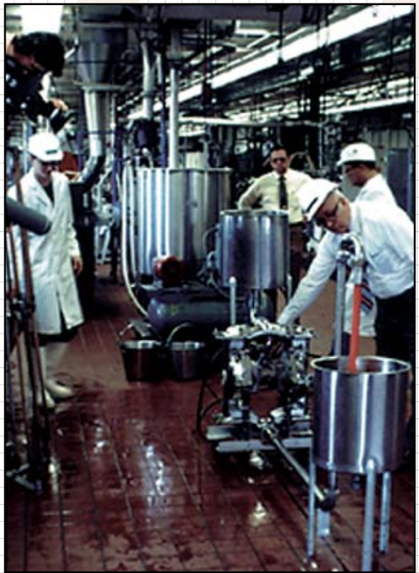
USDA certified flap check valve pumps transferring tomato paste at a major university processing facility.
